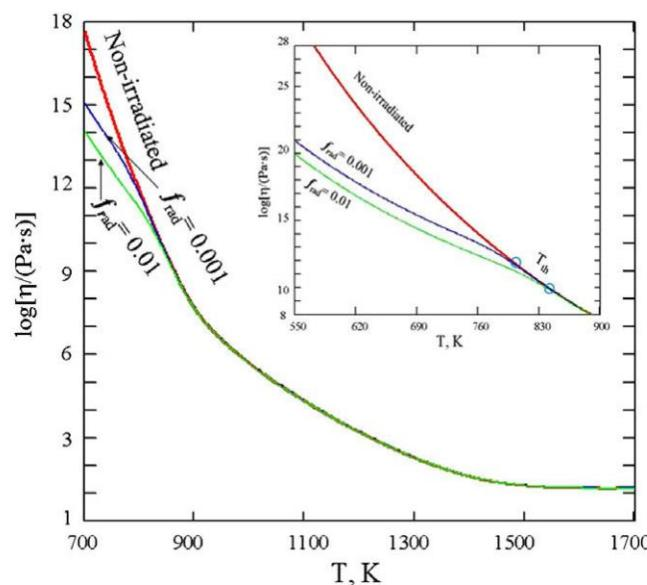
Fig. 9. Viscosities of non-irradiated and electron beam irradiated amorphous soda lime silicate system  $70SiO_221CaO9Na_2O$  as a function of temperature for two dimensionless electron flux densities ( $f_{rad} = \alpha_e I_e$ ) 0.01 and 0.001.
