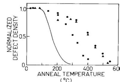
Fig. 7. 10 min isochronal annealing curves for (●) 16.5% densified Suprasil, 1, 76 Mrad irradiation, (▲) 16% densified Suprasil W1 76 Mrad irradiated and (■) PECVD oxide, 10% densified, 20 Mrad irradiated. The solid line shows the annealing curve for  $E'_1$  defects in undensified a-SiO<sub>2</sub>.
