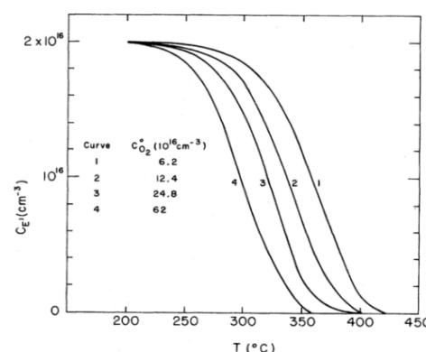
FIG. 10. Plot of  $E'$  concentration  $C_{E'}$ , vs temperature for several different initial concentrations of  $O_2(C_{O_2}^0)$ , from Eq. (4). Other parameters are as given in text.
