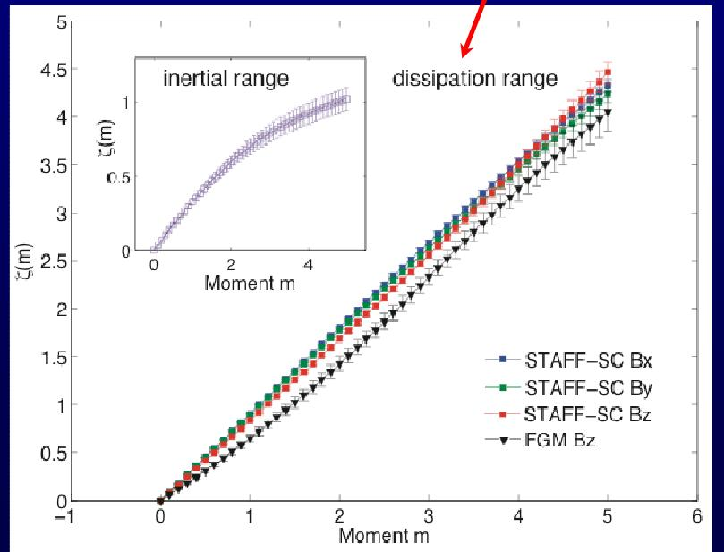
Evidence of monofractality (self-similarity) at sub-proton scales, while MHD-scales are multifractal (intermittent)
