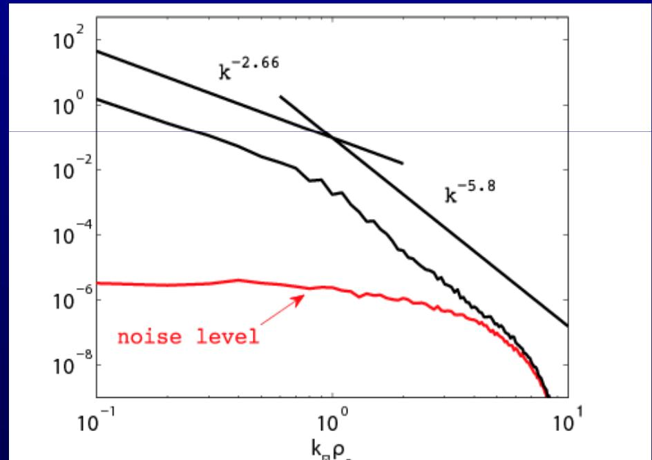
Figure 5. Spectrum of magnetic fluctuation  $|\delta B|^2 / |B_0|^2$  in the perpendicular direction  $k\rho_{e\perp}$ . The noise level curve is in red. The power-law best fits are superimposed.
