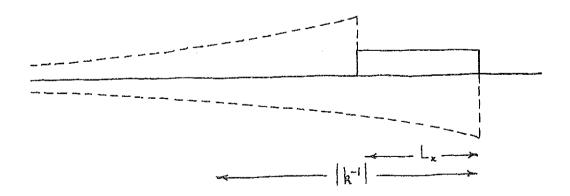
In this limit the e-folding decay scale of the Rossby waves,  $|\mathbf{k}^{-1}|$ , is much longer than the width scale of the wind stress,  $L_{\mathbf{x}}$ ; that is,
