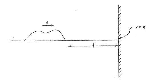
interior. Subsequently, a packet of Kelvin waves leaves the locally forced region and travels toward the eastern ocean boundary. Such a packet is pictured in the diagram. Let that packet be described by
