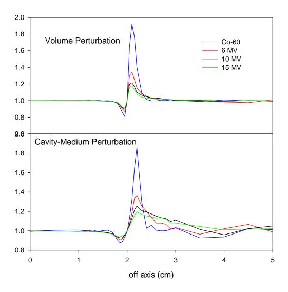
Perturbation factors according Bouchard Radiation: Co-60; chamber radius: 2 mm; length: 10 mm
