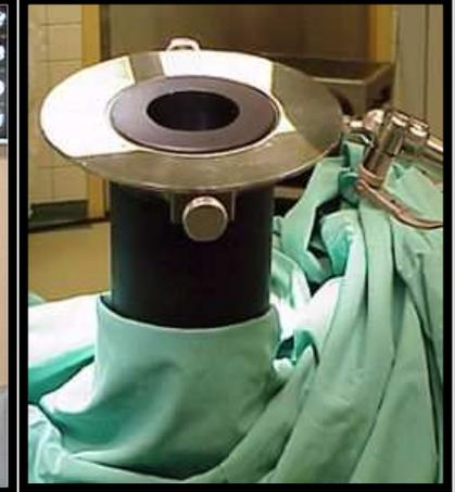
IOERT dedicated, selfshielded, mobile, electron linear accelerator available when needed in a standard operating room, **SOFT DOCKING system**
