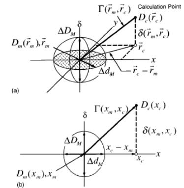
FIG. 2. Geometric representation of dose distribution evaluation criteria using the combined ellipsoidal dose-difference and distance-to-agreement tests. (a) Two-dimensional representation. (b) One-dimensional representation.
