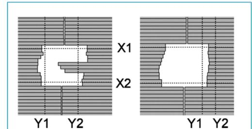
FIG. 3. Two examples of corrupted segments (control points) from a step-and-shoot IMRT plan. Due to a network transfer error, leaf positions of the next segment were used, while jaw positions were correct. MLC leaves are displayed in gray and jaw positions are indicated with dashed lines.
