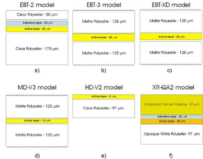
Figure 1. Diagram of the Gafchromic™ film structure/dimensions: (a) EBT2 (b) EBT3 (c) EBT-XD, (d) MD-V3, (e) HD-V2, and (f) XR-QA2 film model.
