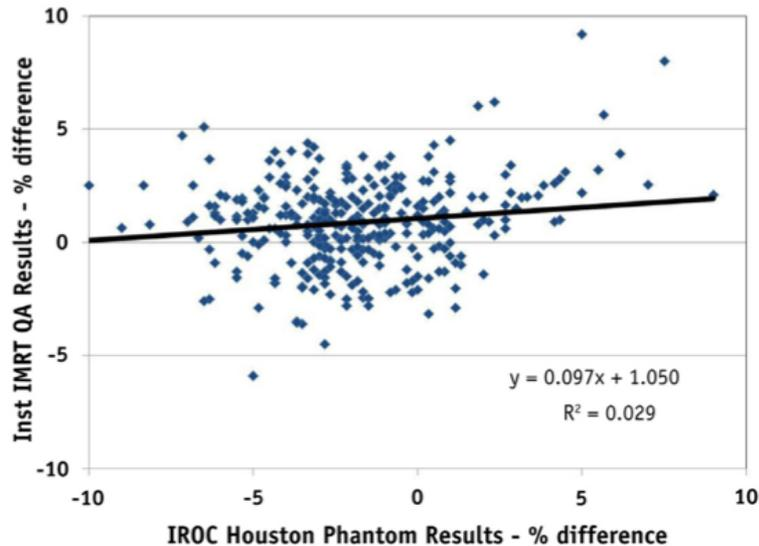
**Fig. 3.** Percent differences between dose measurements and treatment planning system calculations for institutional IMRT QA compared with the TLD in the IROC Houston phantom. The linear trend line should ideally have a slope of 1 but instead is nearly flat. IMRT QA = intensity modulated radiation therapy quality assurance; IROC = Imaging and Radiation Oncology Core; TLD = thermoluminescent dosimeters.
