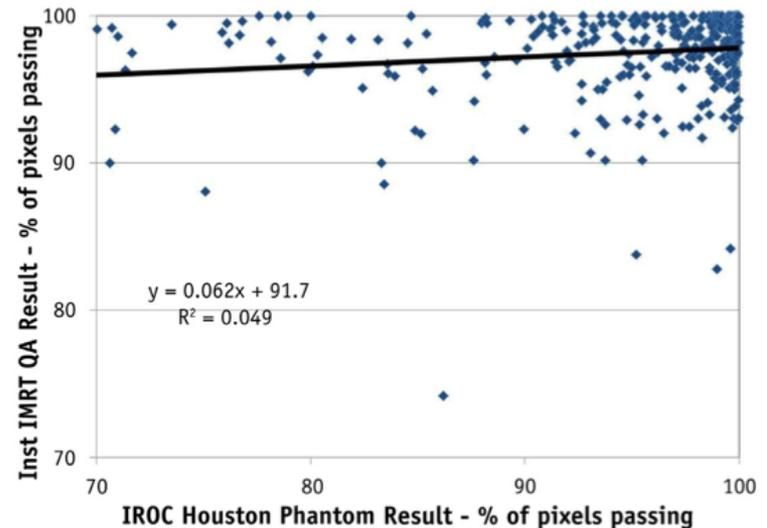
**Fig. 4.** Percent of pixels passing gamma for institutional IMRT QA compared with the IROC Houston phantom films. The linear trend line should ideally have a slope of 1, but instead is nearly flat. IMRT QA = intensity modulated radiation therapy quality assurance; IROC = Imaging and Radiation Oncology Core.
