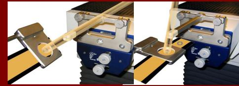
Ball Centroid: Row = 62.22, Column = 59.38 Cone Centroid: Row = 60.87, Column = 60.66 Distance = 1.86 pixels, 0.35 mm
