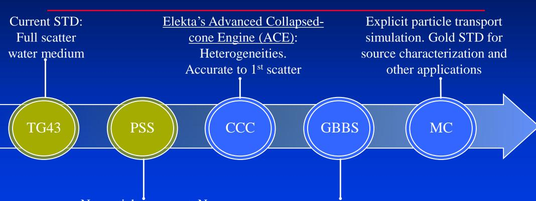
No particle transport. No heterogeneity, shields. Primary can be used in more complex dose engine
