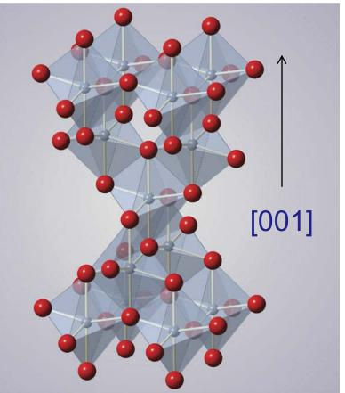
tetragonal, anisotropic unit cell network of corner-sharing or edge sharing TiO<sub>6</sub> octahedra
