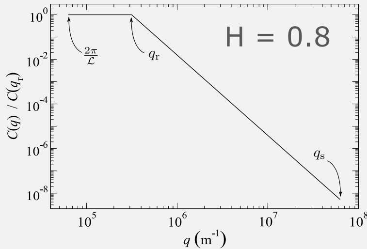
$$L_{\text{sys}} = 0.1 \text{ mm} ; \text{rms-}h = 0.7 \text{ } \mu\text{m}$$
