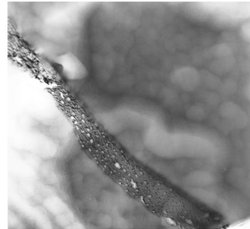
He bubbles on grain boundaries can cause severe embrittlement at high temperatures (S. Zinkle, ORNL)
