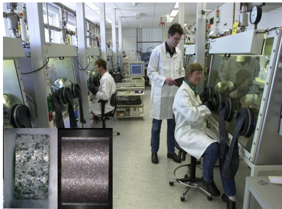
NRG's actinides laboratory; inset shows examples of experimental fuels for incineration of plutonium for the OTTO and FP6 experiment LWR Deputy, respectively; Netherlands
