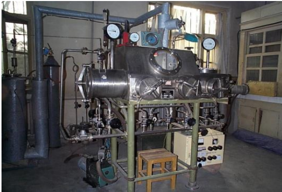
High temperature sodium static test facility for corrosion studies, CEFR, China
