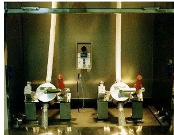
Capsule send and receive stations for ETR-2, Egypt
