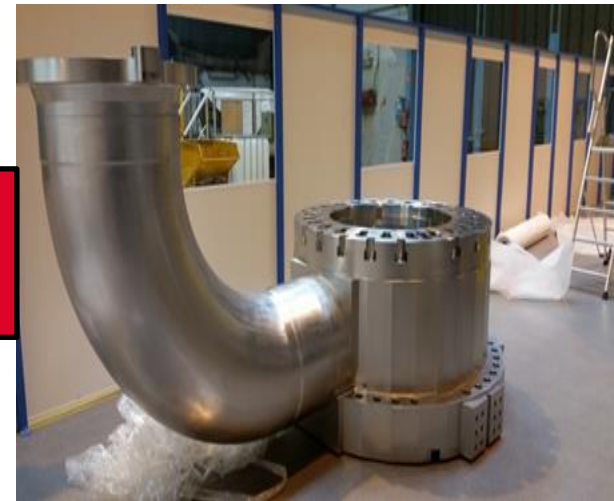
Main water box with primary system connection
