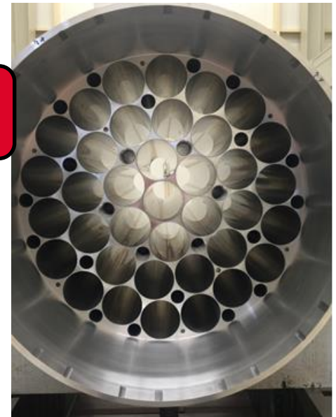
Rack for fuel elements
