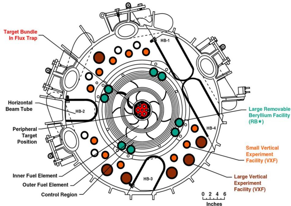
Cross section of HFIR, showing experiment positions
