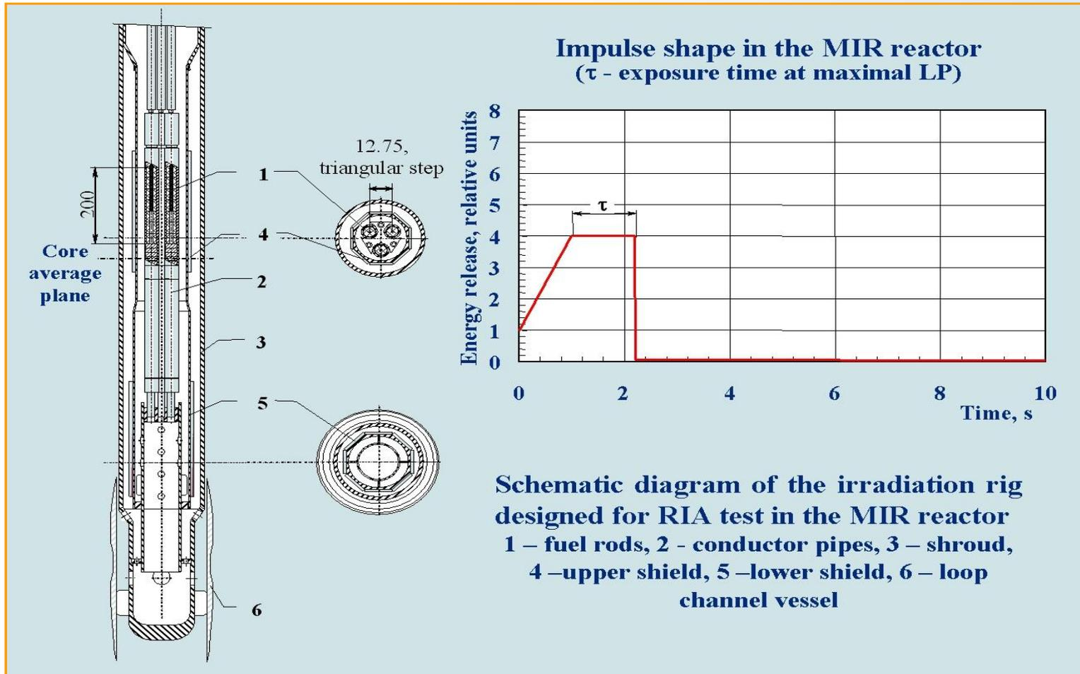
Technique for simulation of reactivity inserted accident (RIA)
