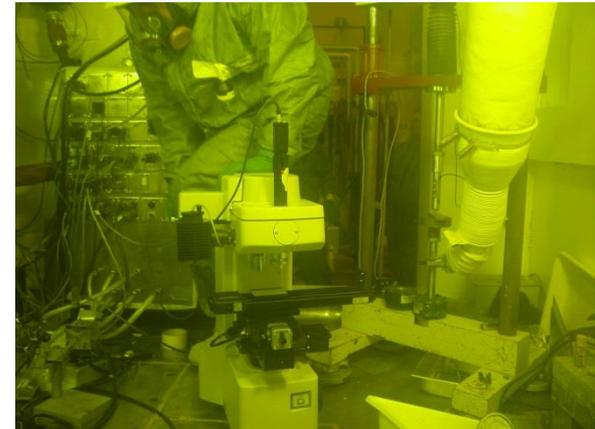
In-cell hardness testing, IMET
