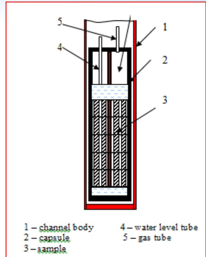
Capsule for irradiating vessel steel samples in boiling water
