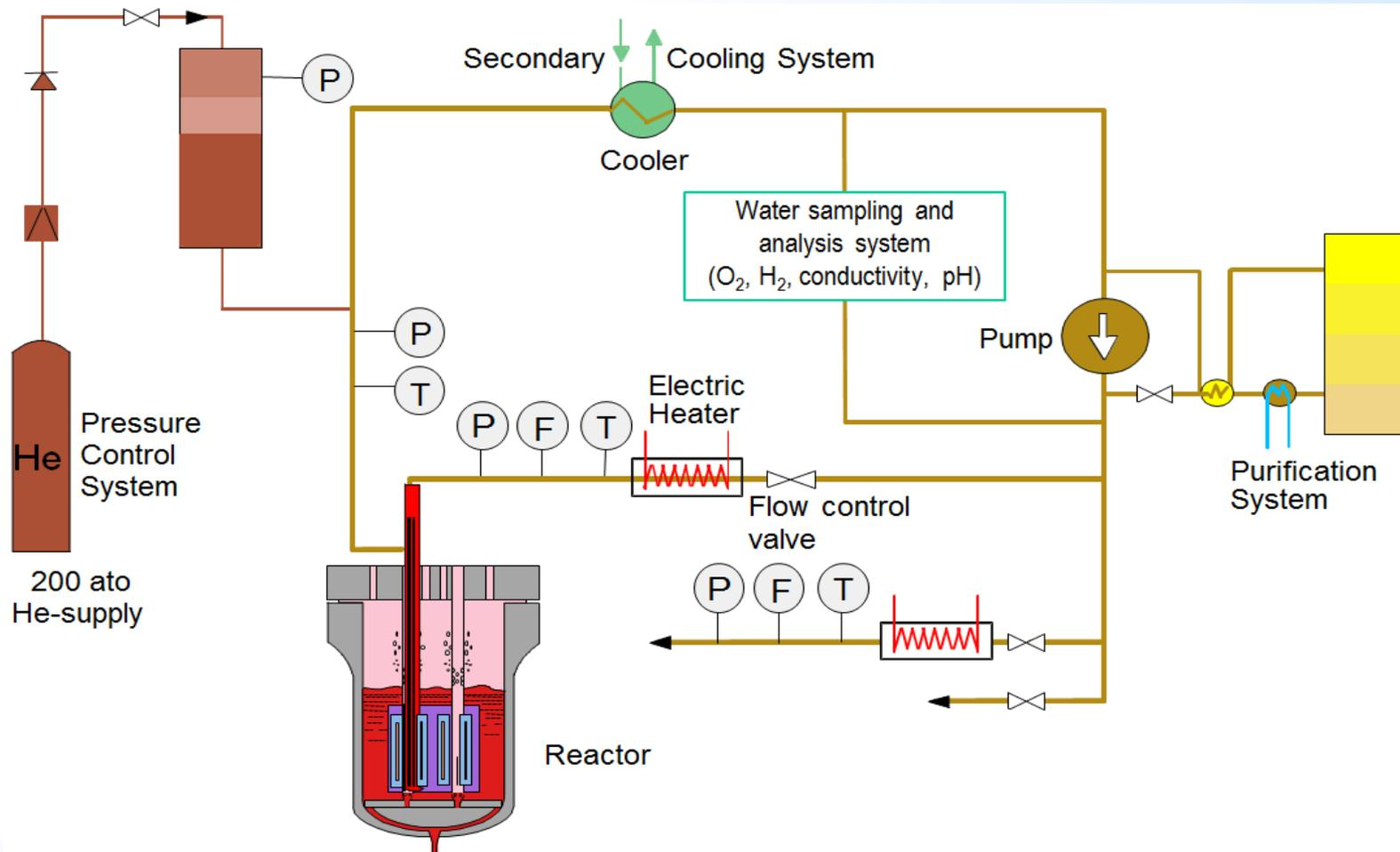
Schematic of a HBWR steady state loop system - can have up to 10 loop systems
