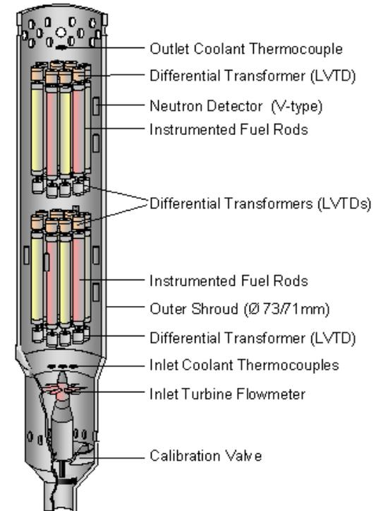
**HBWR irradiation test rig for instrumented fuel rods**
