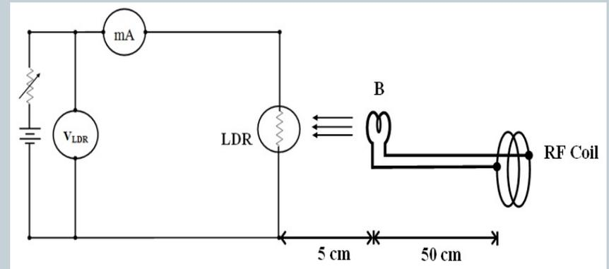
**Figure 3:** Experimental setup for RF power measurement.
