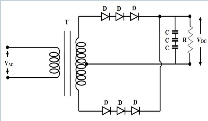
**Figure 2:** Circuit diagram of 1 kV DC power supply.  $T = 100$  VA Step-Up Transformer;  $D =$  IN 4007, 700 V (PIV);  $C = 330 \mu\text{F}$ , 450 V;  $R = 1.18 \text{ M}\Omega$ .
