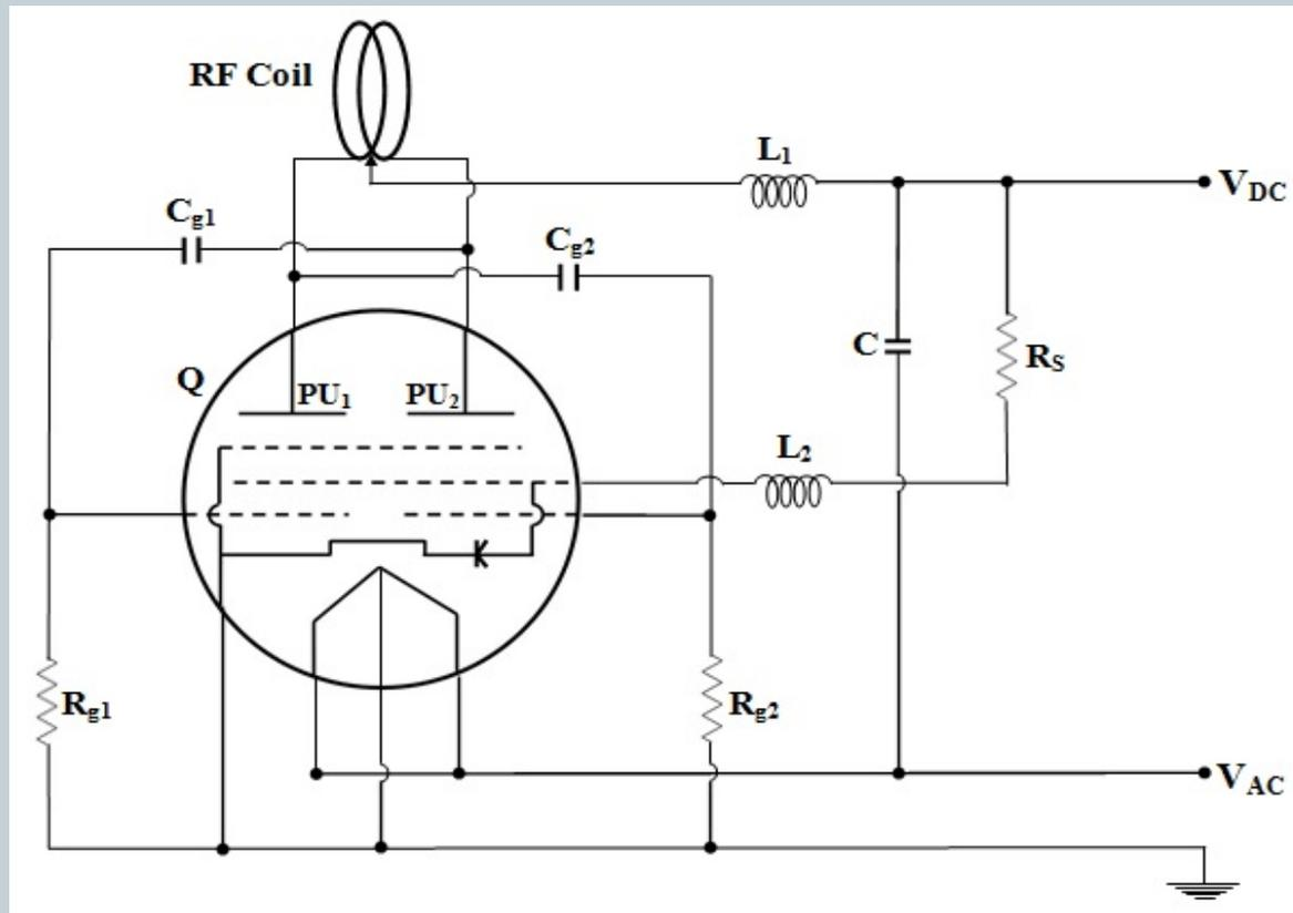
**Figure 1:** Circuit diagram of RF oscillator. Q = 829B/GI30 twin beam-power tetrode; RF Coil: tube diameter = 0.6 cm, pitch = 1 cm, coil diameter = 7 cm;  $R_S = 20 \text{ k}\Omega$ , 20 W;  $R_{g1} = R_{g2} = 6.8 \text{ k}\Omega$ , 1 W;  $C_{g1} = C_{g2} = 1 \text{ pF}$ , 1 kV;  $C = 50 \text{ }\mu\text{F}$ ,  $L_1 = 586 \text{ }\mu\text{H}$ ;  $L_2 = 589.5 \text{ }\mu\text{H}$ .
