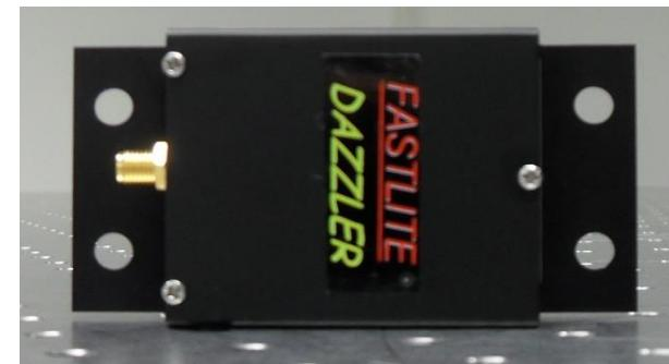
**Acoustic-Optic Programmable Dispersive Filter for spectral amplitude and phase control**
