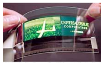
OLED Display Screen (from Universal Display Corp)
