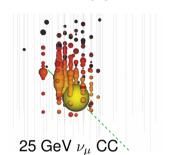
$\begin{array}{c} \text{color} \rightarrow \text{hit time} \\ \text{size} \rightarrow \text{hit charge} \end{array}$
