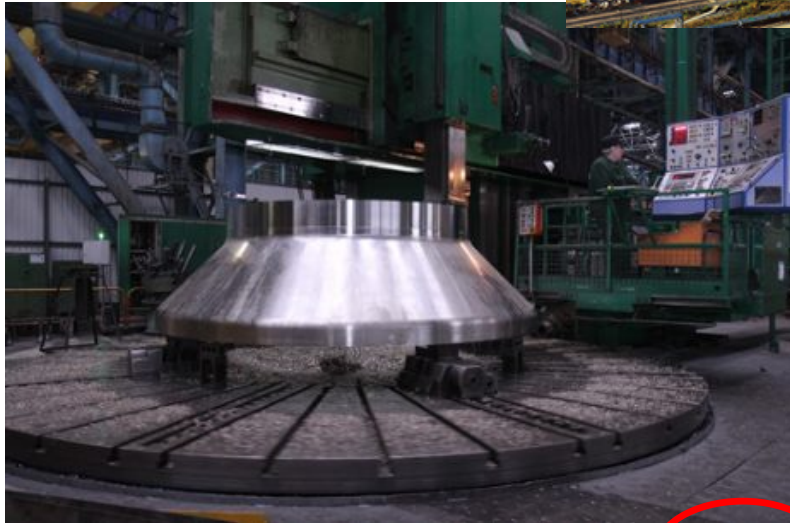
The upper part of the reactor vessel for MBIR (Image: AEM-Technology)
