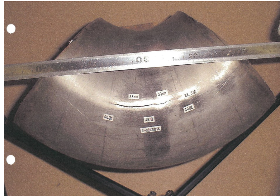
Thin-walled piping after vibration test simulating severe earthquake load
