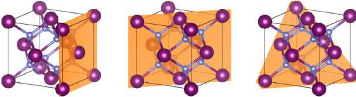
Uranium dioxide has the cubic fluorite crystal structure, space group  $Fm\bar{3}m$ , ( $a = 5.469\text{\AA}$ )
