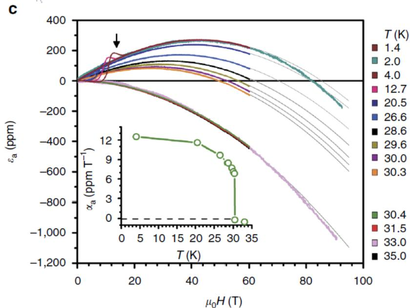
The unusually low thermal conductivity of  $\text{UO}_2$  cripples its performance as a fuel in nuclear reactors. Here we uncover first-order coupling between the magnetism in U-atoms and lattice degrees of freedom that could be the origin of scattering of phonons against spin fluctuations dressed with dynamic Jahn-Teller oxygen modes well above  $T_N$ . These effects should be explored further.
