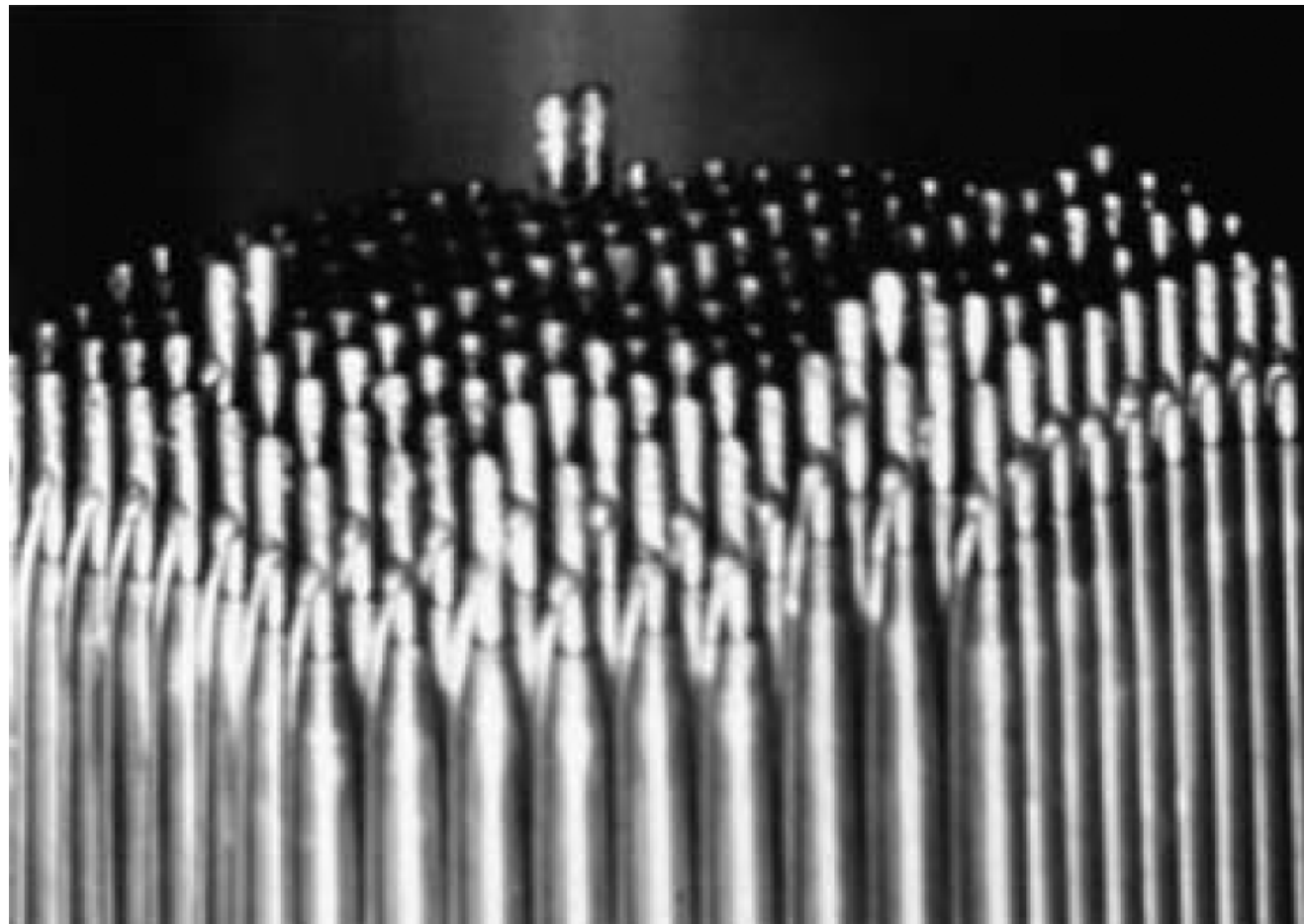
D-9 stainless steel austenitic 15Cr-15Ni stabilised with Ti
