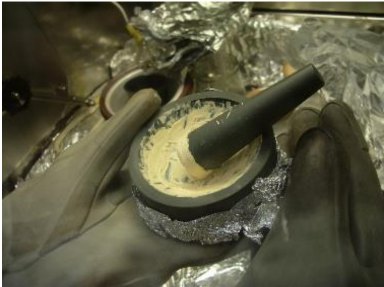
Grinding the mixture into a mortar inside glove-box
