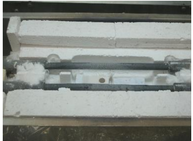
Sintering in air inside glove-box at temperature 1500°C
