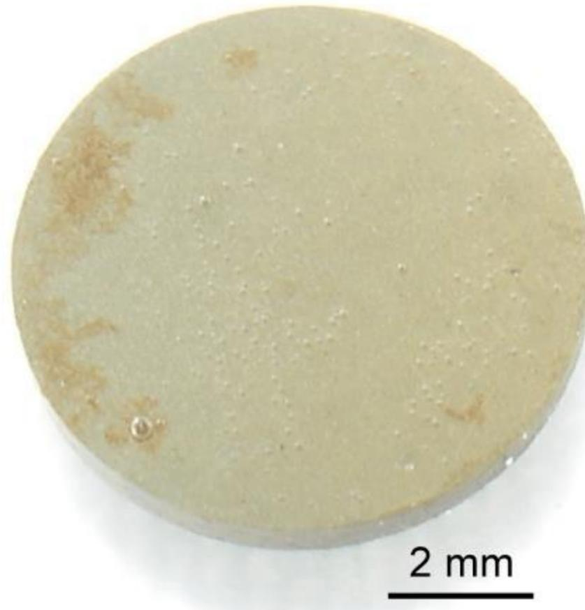
Cubic zirconia (Zr,Gd,Pu)O<sub>2</sub> doped with **9.9 wt. % Pu-238**. Synthesized in 2000.
