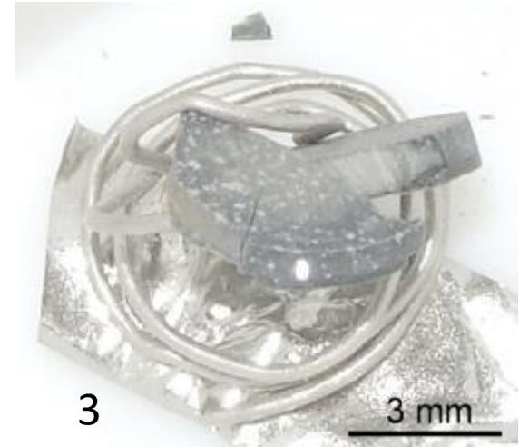
Pellet of single-phase  $^{238}\text{Pu}$ -doped ceramic,  $\text{La}_{0.9}\text{Pu}_{0.1}\text{PO}_4$ , at accumulated dose approximately  $10^{26}$  alpha-decays/m<sup>3</sup>:
