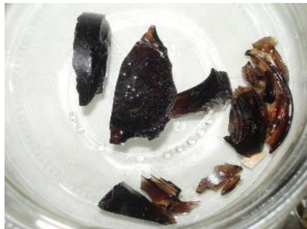
**Sample of SON-68 glass doped with 0,4 macc.%  $^{238}\text{Pu}$  right after synthesis**
