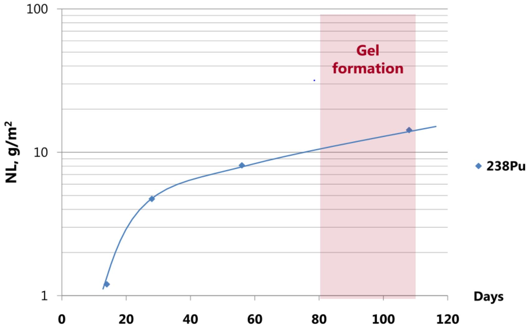
$^{238}\text{Pu}$  normalized mass loss (90C, static, distilled water)
