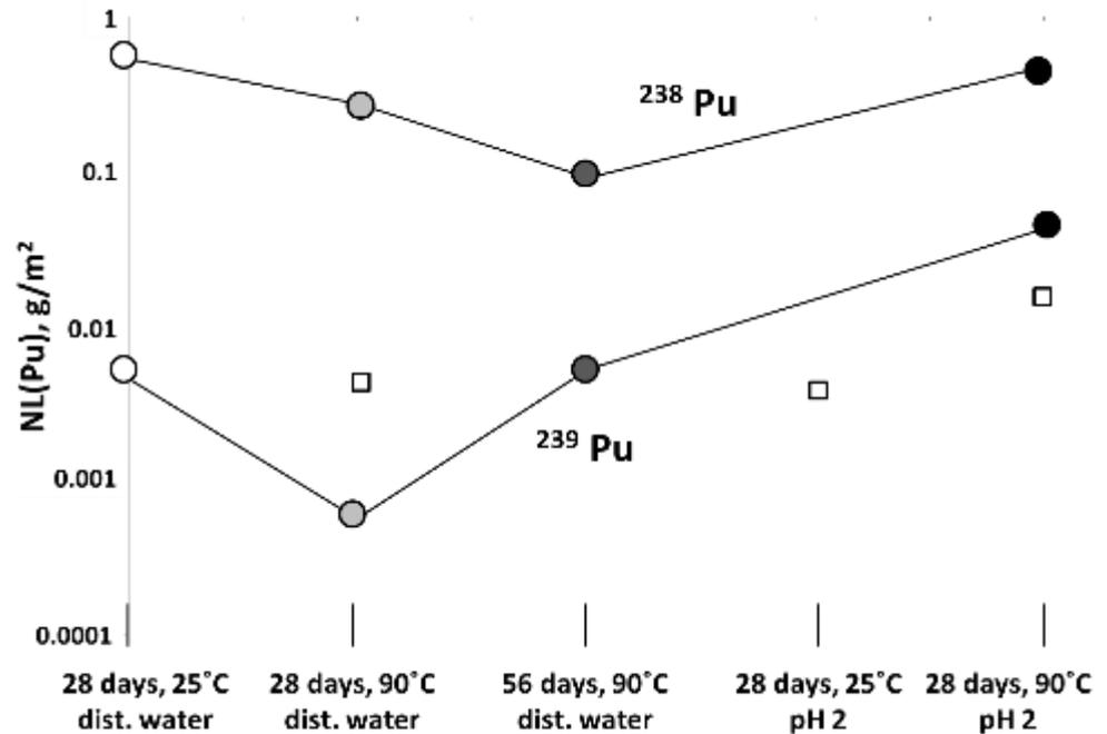
Results of  $\text{PuO}_2$  static leach tests: ○ and ● – polycrystalline samples (the same pellet was used in different tests); □ – single crystals (only separate fresh samples for each test)
