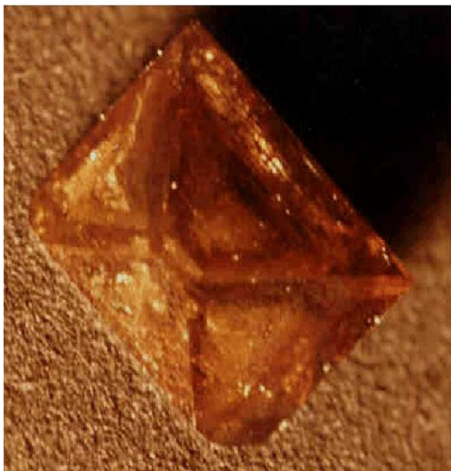
. Fig. 11 The photographs of zircon crystals ( \text{ZrSiO}_4\text{:Pu} ) not activated by rare-earth ions.
