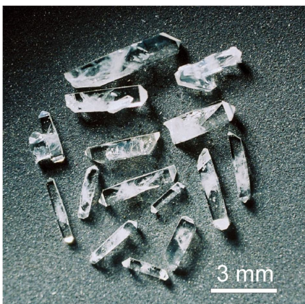
. Fig. 12 The photographs of zircon crystals ( \text{ZrSiO}_4\text{:Pu, In} ) not activated by rare-earth ions
