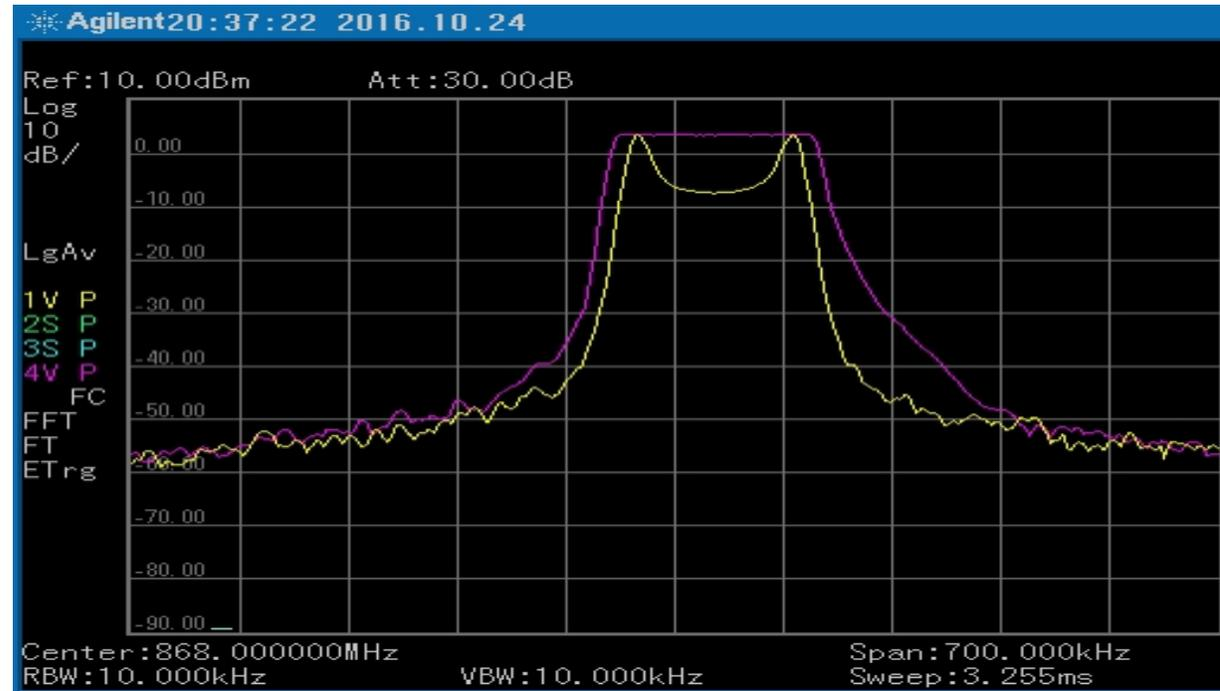
Flat top LoRa spectrum implies a more efficient spectrum usage as compared with the two peaked FSK. Output power is the same, bandwidth is 125 kHz
