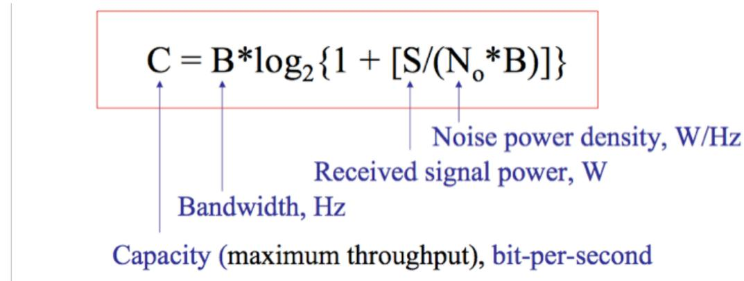
The diagram shows the equation C = B \* log2 {1 + [S / (No \* B)]} enclosed in a red box. Below the box, four blue arrows point upwards to the variables in the equation: C, B, S, and No. Each arrow is accompanied by a label: 'Capacity (maximum throughput), bit-per-second' for C, 'Bandwidth, Hz' for B, 'Received signal power, W' for S, and 'Noise power density, W/Hz' for No.
