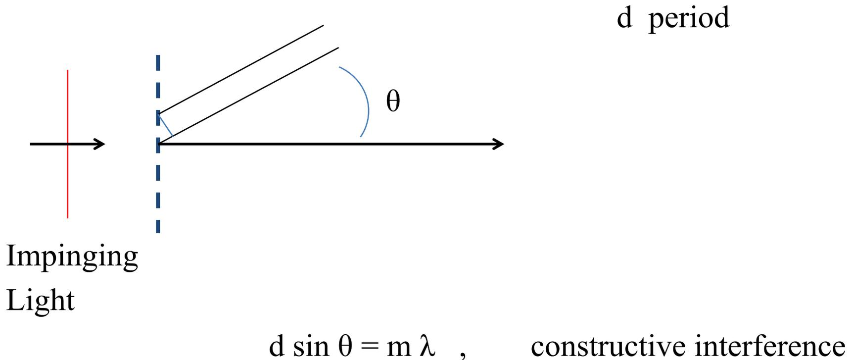
Laser beams of **different frequencies** are sent on a low frequency diffraction grating and **diffraction orders** of the different lasers are produced.
