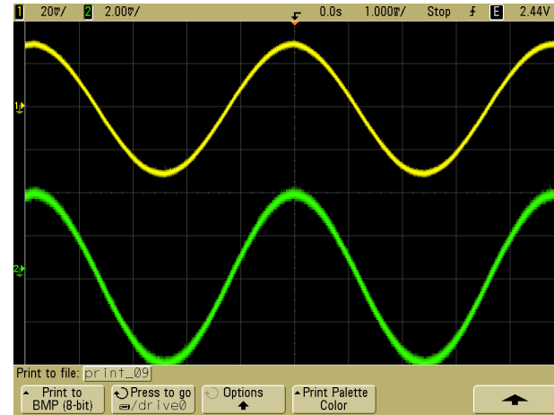
Green trace – current signal Yellow trace – voltage signal
