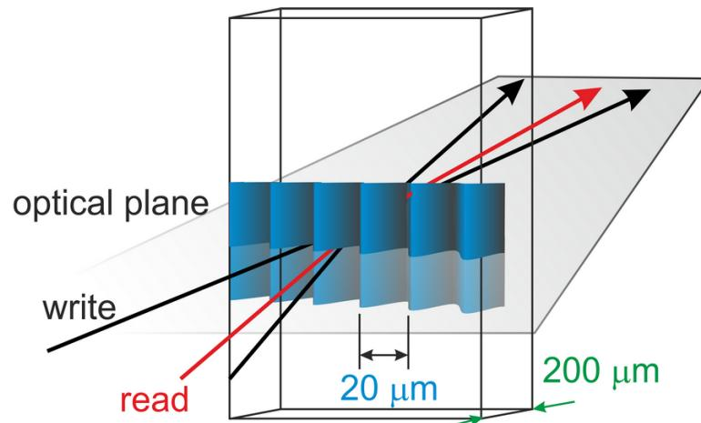
**IR-TDFRS – InfraRed -Thermal Diffusion Forced Rayleigh Scattering**
