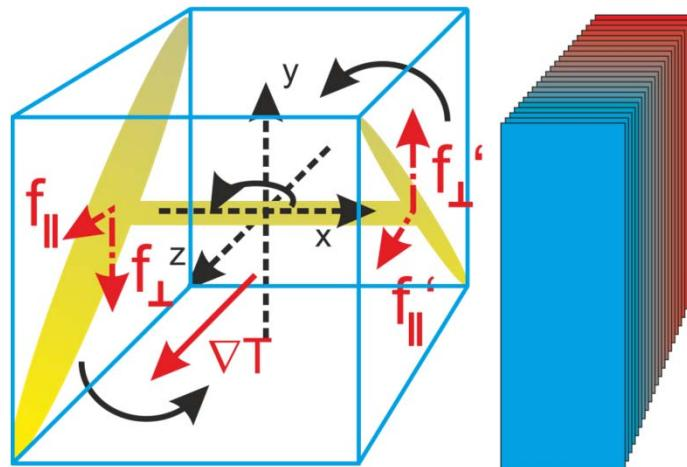
If two ellipsoidal blades with opposite orientation angles connected by a rigid bond, which is perpendicular to an external thermal gradient they can rotate.
