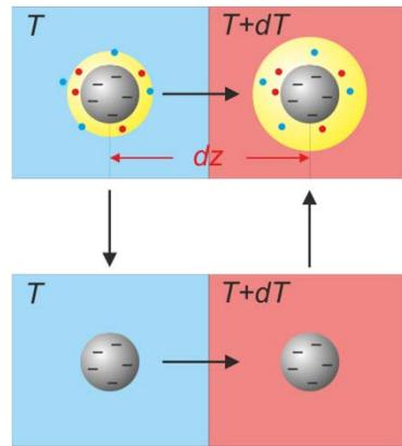
$$\begin{aligned} \mathcal{F} \cdot dz &= -(-dW^{(dl)}(T) + dW^{(dl)}(T + dT)) \\ &= -dT \frac{dW^{(dl)}(T)}{dT} \end{aligned}$$
