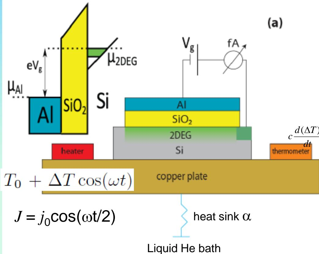
$$i(t) = \frac{\partial \mu}{\partial T} \Delta T C_0 \sin(\omega t)$$
