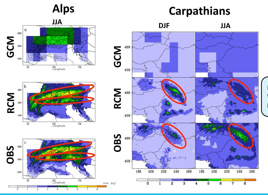
RCM ensemble is able to capture the topographically-induced precipitation patterns.
