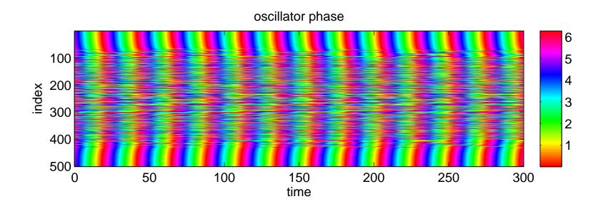
Even though oscillators are identical and coupled in highly-symmetric way, they split into synchronous and asynchronous groups.
