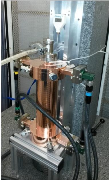
Accelerating structures are tested in specific test stand
