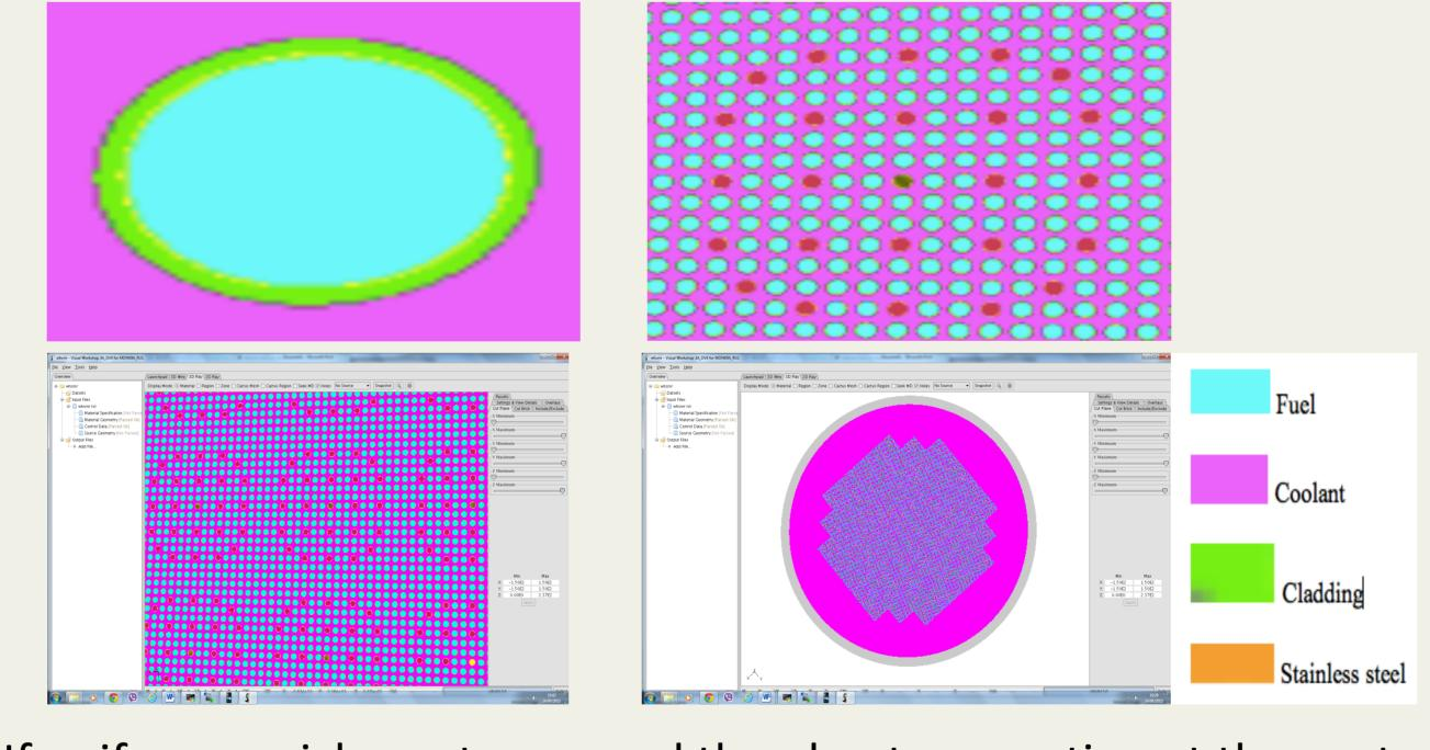
If uniform enrichment was used then heat generation at the centre would be very high compared to the boundary and would generate hot spots near the centre<sup>4</sup>.
