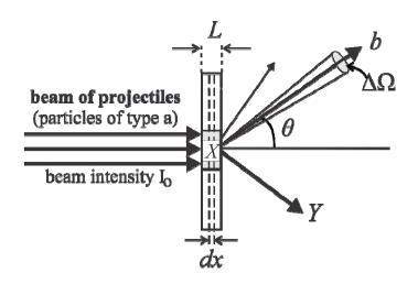
$$\sigma = \frac{reactions \ per \ time}{(projectiles \ per \ area \ per \ time) \times (target \ nuclei)}$$
