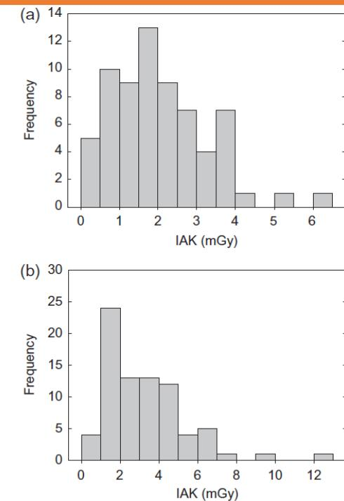
Figure 3. Measurement result as IAK in intraoral dental radiography devices under (a) low dose modes and (b) high dose modes.
