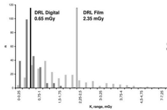
Figure 2. Distribution of  $K_i$  for minimum exposure settings (incisors), for film and digital imaging.
