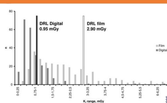
Figure 3. Distribution of  $K_i$  for average exposure settings for film and digital imaging.
