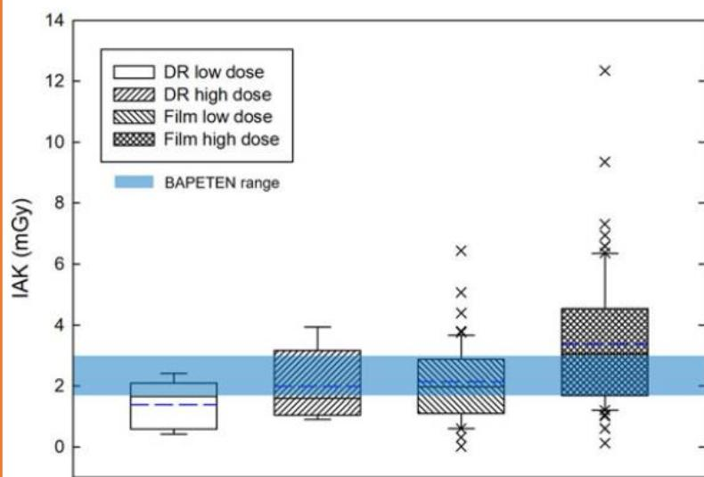
Figure 5. Incident air kerma (IAK) of intraoral devices by modes and image receptors used.
