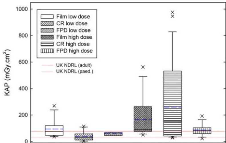
Figure 6. Air kerma area product (KAP) of the panoramic devices by modes and image receptors used.
