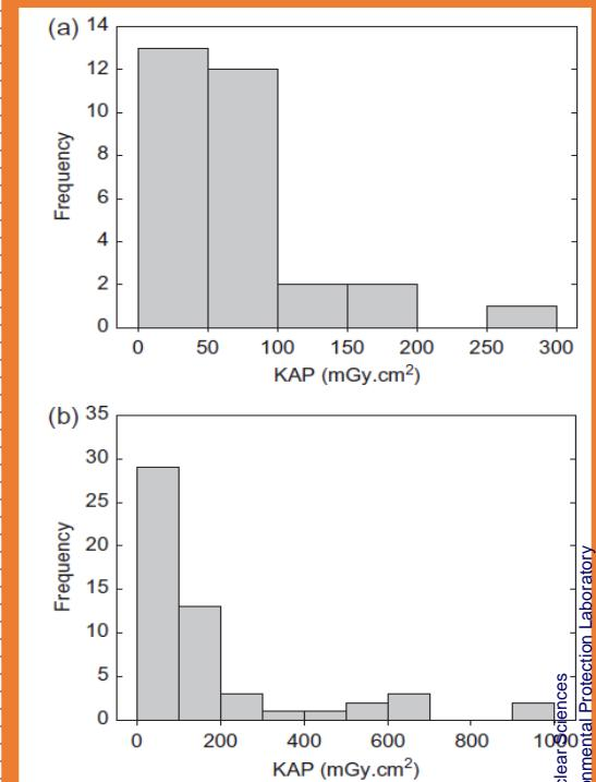
Figure 4. Measurement result as KAP in panoramic dental radiography devices under (a) low dose modes and (b) high dose modes.
