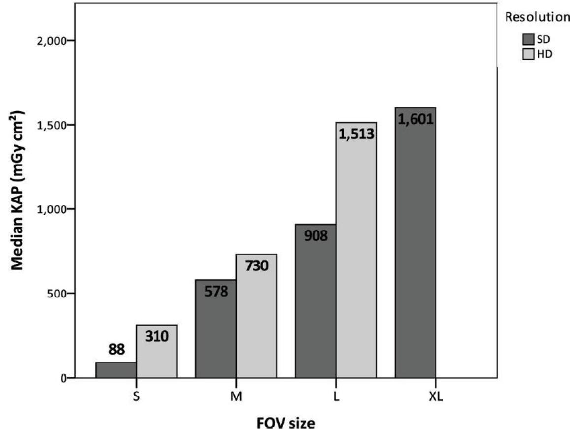
Figure 7 Median values of air kerma-area product ( $\text{mGy cm}^2$ ) for different FOV sizes and two resolution modes—HD (voxel size  $<0.2\text{ mm}$ ) and SD (voxel size  $\geq0.2\text{ mm}$ ) in 15 different institutions from four countries. FOV, field of view; HD, high definition; SD, standard definition.
