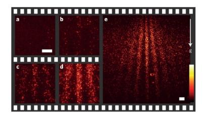
Modern *which-path* experiment with stochastically arriving phthalocyanine (PcH2) molecules (one at a time)
