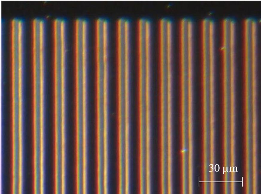
Optical image of a gold wires array
