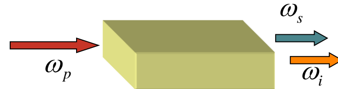
Parametric down-conversion (PDC)
