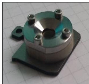
Ultralene membrane (4 \mu ) for Omicron compatible liquid sample cells, KMC-1, HZB
