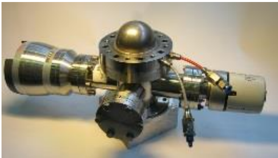
KMC-2 at BESSY-II: custom-built Beryllium dome furnace with double sided borolectric® heater reaches temperatures up to 1000 °C in vacuum (< 10 -9 mbar)
