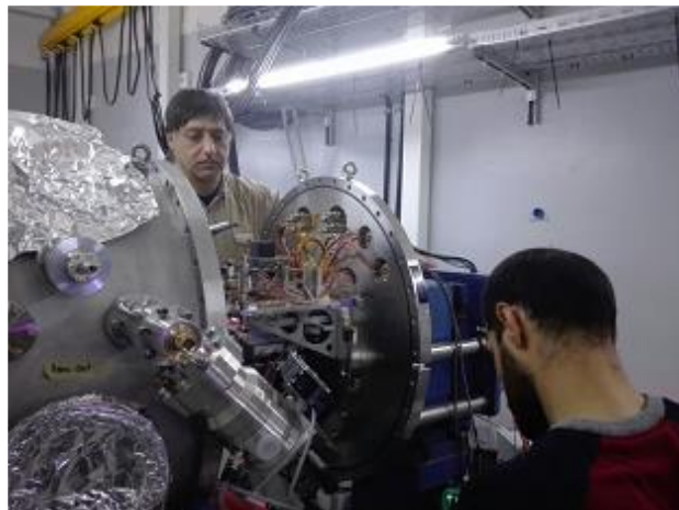
Motors and wiring of the DCM
