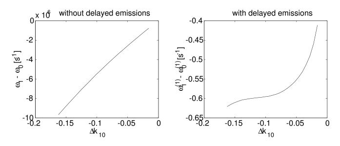
1.Relation between the separation of the first static multiplication eigenvalues and the separation of the first time eigenvalues.
