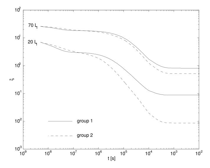
6.Evolution of the spatiality parameter  $\xi$  for two subcritical systems having  $\Delta k/k = -1.4114\beta$ . The reference  $\Psi$  is the final flux distribution.
