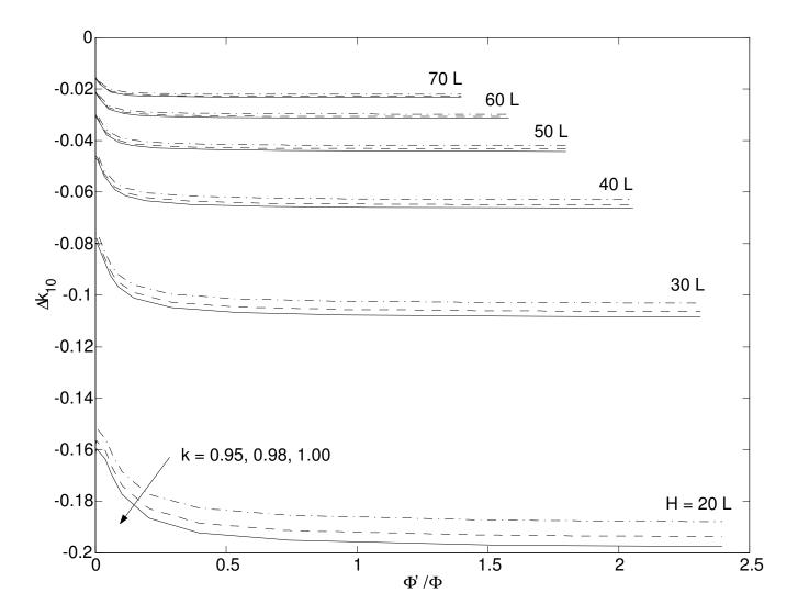
4. Eigenvalue separation for different values of the greyness of the control device and of the physical dimensions of the system.
