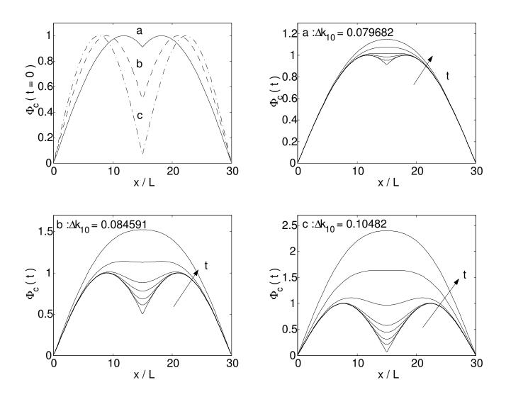
5.Spatial evolution in initially critical systems with different eigenvalue separations. The top left graph reports the initial flux distributions for three values of the greyness of the control device.
