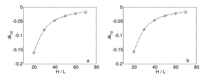
2.Eigenvalue separation for critical and subcritical systems. The circles indicate results for the homogeneous system and crosses for a system with an absorber that introduces a change in k of -500 pcm. Graph (a) on the left refers to the case in which the homogeneous system is critical, while graph (b) refers to the case in which the homogeneous system is subcritical (k = 0.98).
