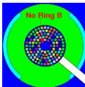
Figure 3. Sub-critical configuration without fuel rods on ring B
