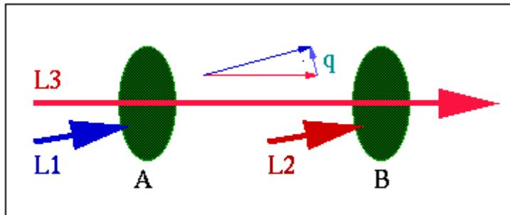
‘A’ and ‘B’ are two condensates, L1 and L2 are pump lasers, L3 is a common entangling probe laser. Both the pumps have same wave vectors  $k_1$ , probe’s wave vector  $k_2$ . The probe is red detuned from the pumps. The laser are in Bragg resonance with a particular momentum mode  $q$  of both the condensates.
