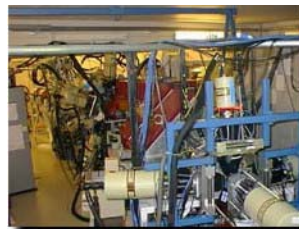
Light charged-particle detector Microball – 96 \text{ CsI} with photo diodes
