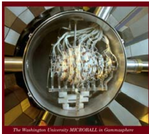
Light charged-particle detector Microball – 96 \text{ CsI} with photo diodes
