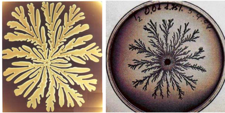
FIGURE 3.12. On the left the viscous fingering effect made by injecting air in a glycerin solution. On the right growth of bacteria colonies (Guyon and Stanley, 1991).
