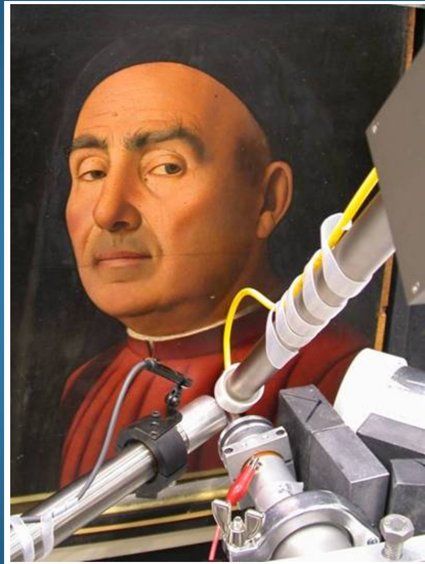
Differential PIXE and PIGE analysis of the "Ritratto Trivulzio" by Antonello da Messina
