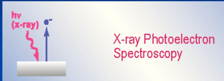
Surface of the sample is excited with X-rays, photoelectrons are emitted from the atoms near the surface. Chemical bonding information may be determined.
