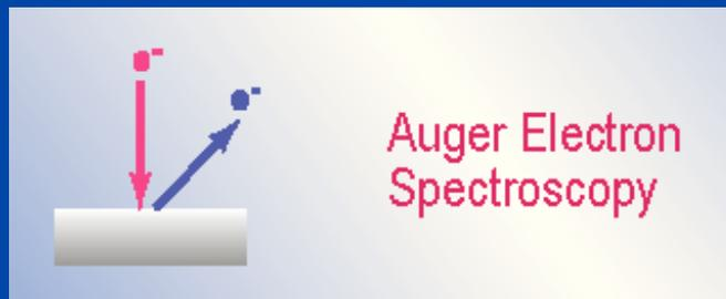
Focused electron beam produces Auger electrons with discrete energies, specific to each element. (Escape depth  $\approx 10 \text{ \AA}$ ) (Sputtering is needed.)
