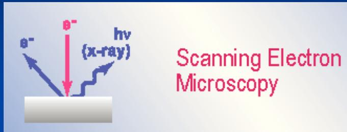
Finely focused  $e$ -beam is rastered over the sample surface, its image is formed from secondary electrons and photon emission. Energy dispersive X-ray (EDX) spectroscopy is also possible - elemental quantification.
