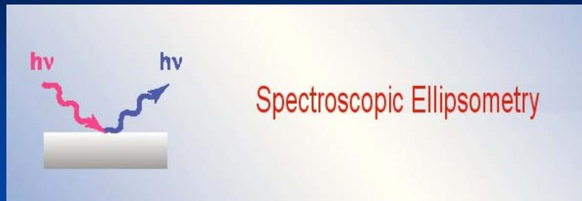
Polarized light scattered on the sample surface, complex refractive index can be determined, layer structure can be obtained. *Good depth scale!*
