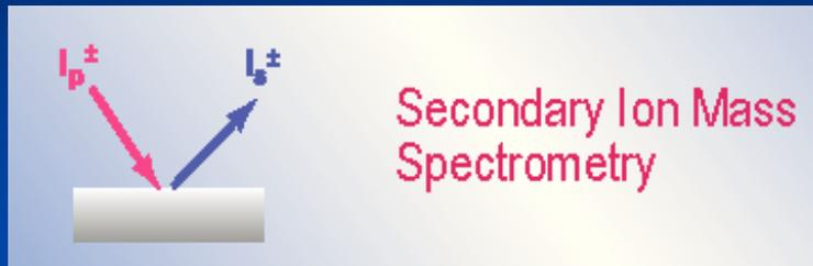
An energetic ion beam is used to sputter atoms from the surface. Secondary ions emitted are mass analyzed.
