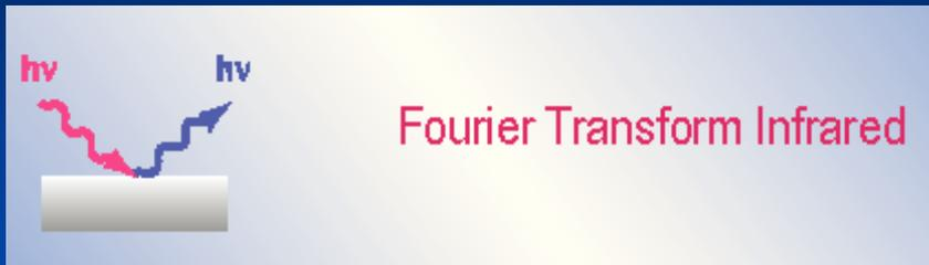
Infrared beam excites the sample, molecular constituents vibrate in the IR regime. The molecules, surrounding environments and concentrations of the oscillating chemical bonds may be determined.
