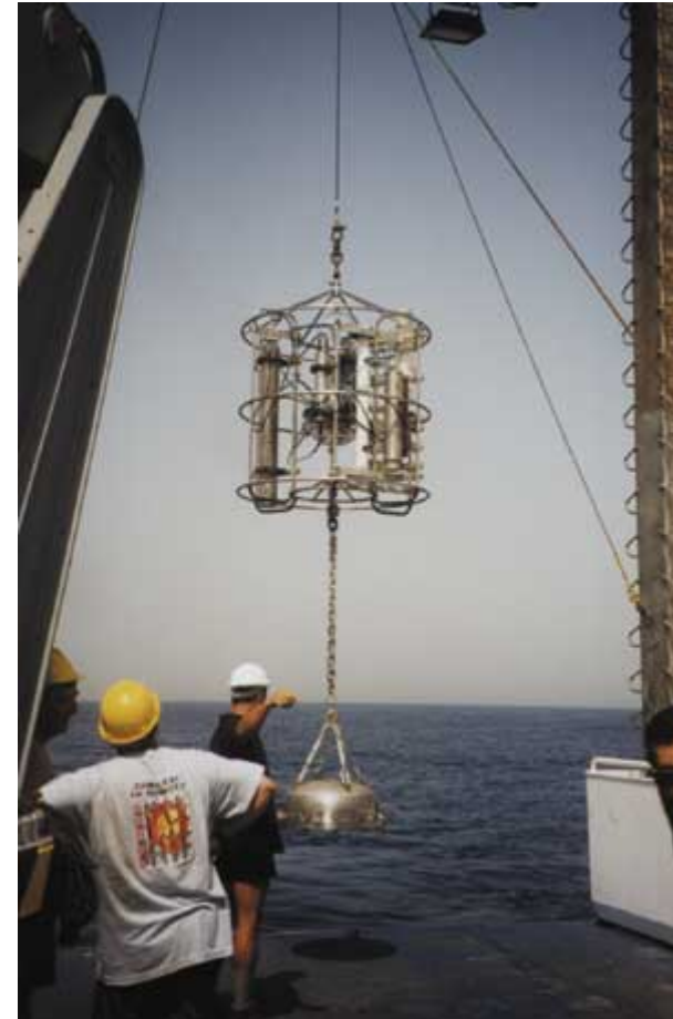
NEMO experiment in Italy. Apparatus to detect the Cerenkov light produced by the passage of neutrinos through water to be installed undersea at a depth of two 5 kilometers .
