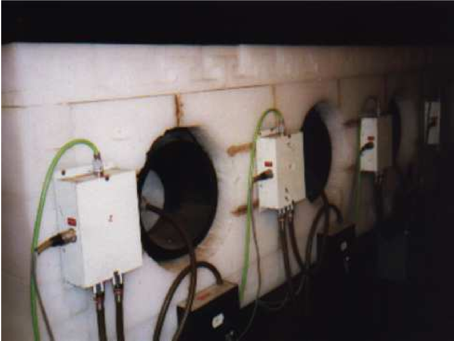
Detail of detectors of neutron monitor. Altogether 8 proportional counters SNM-15 are at Lomnický Štít mountain.
